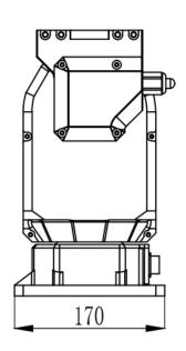
2) Dimension drawing of pan-tilt head roof
