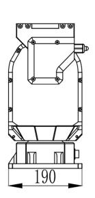
2) Pan-tilt head Roof Dimension Drawing
